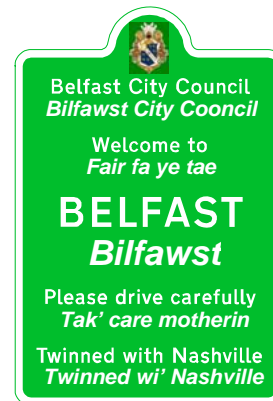
Figure 4 All sign elements in Ulster-Scots (1.9 x 2.7m 150 / 75mm x-height)
